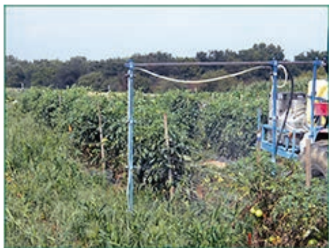
Custom sprayer at the Penn State SE Research Farm, illustrating spraying from multiple angles.
